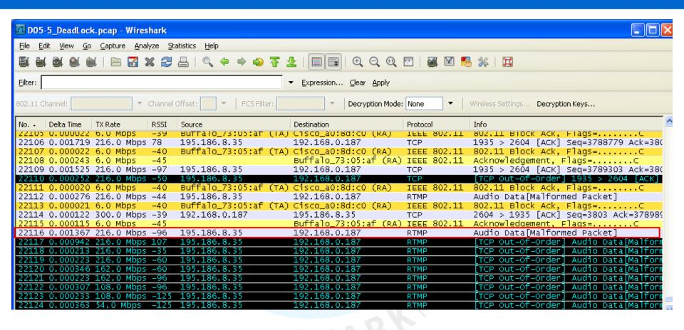
Problem starts at frame # 22116 which is not acknowledged by receiver
