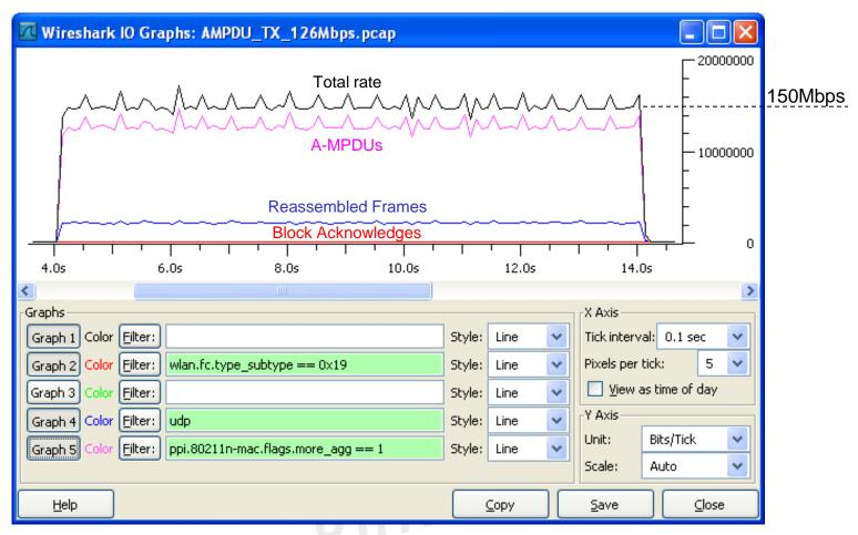
UDP bandwidth measurement with **IPerf** indicates throughput of 126Mbps
