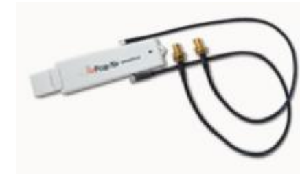
802.11a/b/g/n USB wireless Adapter with two external antennas
